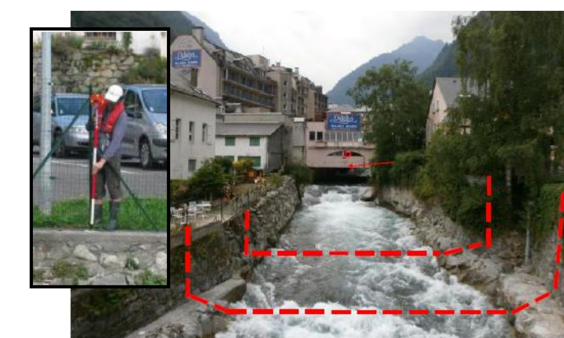
3 : Achieve field topography survey : reference points and bathymetry
